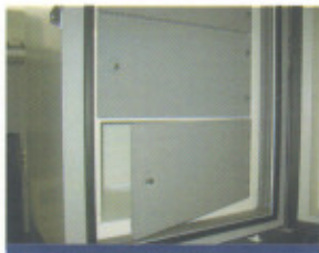
Dual layered air insulated inner doors retain cold air in chamber
