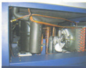
Fluid separator prevents oil from compressors from entering system
